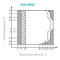
Operating range with heat pump with possible limitation and protection
