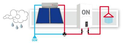
In case of insufficient irradiation and therefore the domestic hot water being modestly pre-heated, the boiler will contribute with the necessary heat to reach the required setpoint temperature.
