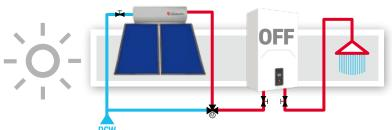
If the sun and the solar system fulfil their "duty", no integration from the boiler will be necessary; the hot water will be conveyed to the tap, without additional devices being required, with the mixing of the thermostatic valves.
