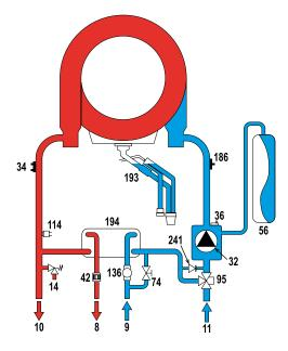
**KEY** DHW water outlet DHW inlet 10 System delivery 11 System return 14 Safety valve 32 Heating circulator 34 36 Automatic air vent
